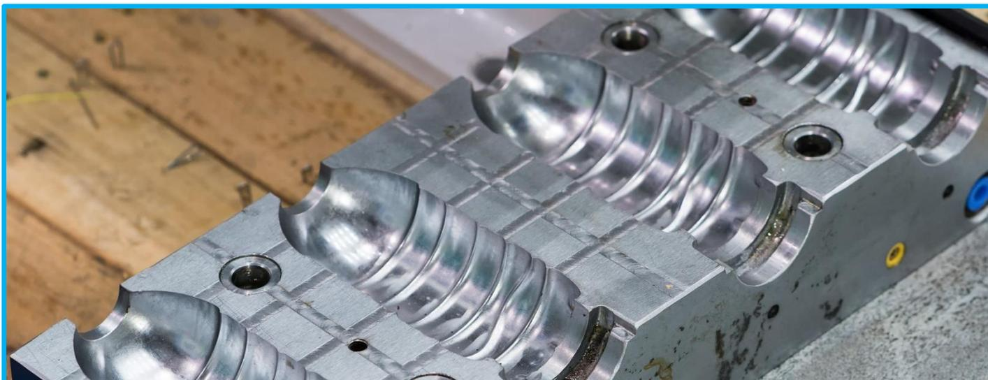
plastic out of the tool, ejector pins or other methods are needed to move through a cavity pushing the part from the cavity.
